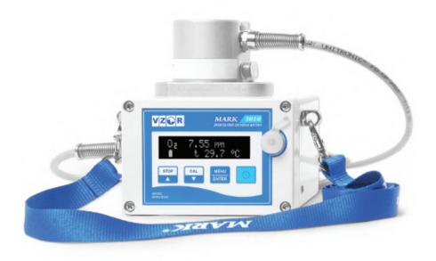
Convenience and accuracy of measurement | Measurement accuracy ±[0,001+1% of measured value], ppm. Ability to work at small flow rates (min. 20 ml/min). Air calibration max. once a month. Routine maintenance once per year. General unit for direct attachment to the process.
